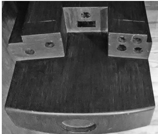
Figure 26 Model of Baoshu Kong Longevity Holes, Quanzhou Maritime Museum
