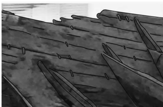
Figure 15 Quanzhou Ship Plank Fastenings, Ribs, and Bulkhead, Quanzhou Maritime Museum
