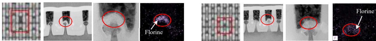
Figure 3. TEM analysis of detected TS open defects.
