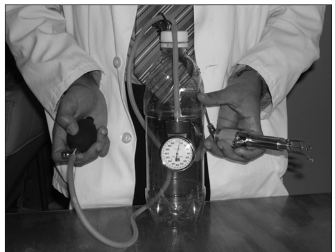
Figure 2: Orbicularis Oculi Pressure Sensor (OOPS).
