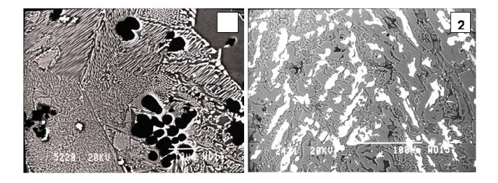
Fig. 1. Backscatter image of the  $Al_{12}$ : $Ru_{11}$ : $Y_{77}$  sample showing dark  $Y_2O_3$  particles,  $\sim Y_{75}Ru_9Al_{16}$  (medium), in a  $\sim Y_{75}Ru_9Al_{16} + Y_3Ru$  (light) eutectic.
