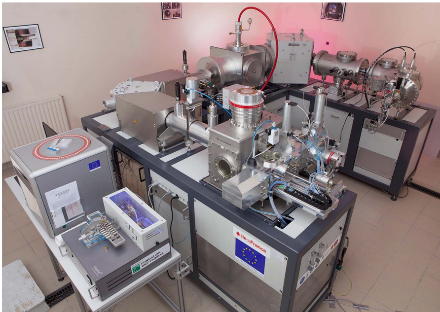
Figure 3. ECHO-MICADAS, the mini radiocarbon dating system at Gif-sur-Yvette, France (photograph: F. Rhodes/CEA).
