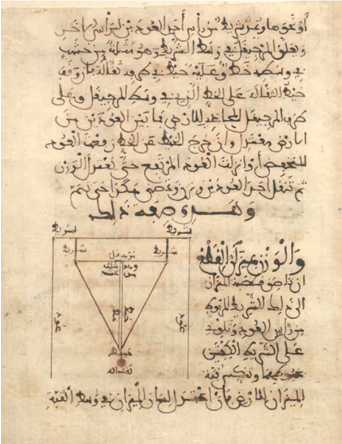
Figure 36 Ibn Luyun’s diagram of a murjiqal, or levelling device (courtesy of the Escuela de Estudios Arabes, CSIC)
