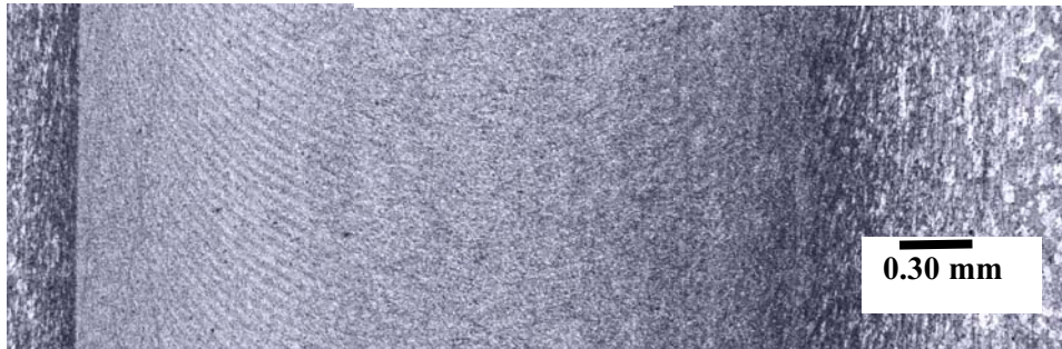
Fig. 1 showing weld path and striations at mid thickness.
