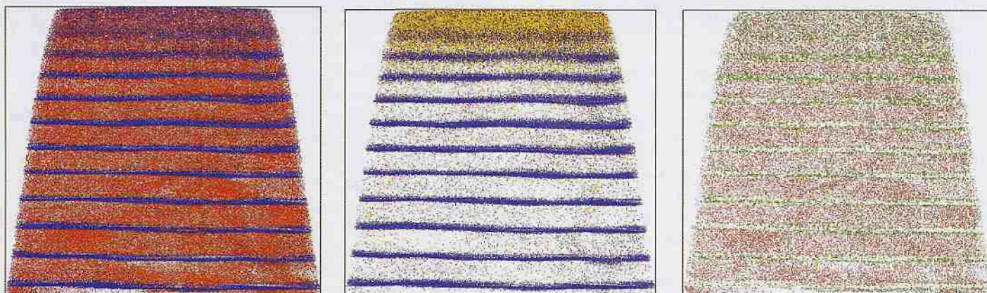
Figure 5, LEAP 3D image of a multilayer stack of PtMn layers with CoFe layers. a) Mn and Co atoms shown to depict the layers. b) Ga shown to depict the ion implantation from the focused ion beam. c) C shown to depict the impurity presence at low concentration and segregation to the CoFe layers. The Mn is shown in red, Co is shown in blue, Ga is shown in gold, and C is shown in green. The layer repeat distance is 12 nm. This image is from the work of Peter Ladwig and Austin Chang of the University of Wisconsin, David Larson of Seagate Recording Technologies and Imago personnel.
