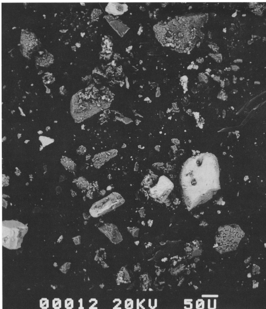
Figure 2. Backscatter electron image from sample 6 after CBD treatment. Elemental composition of bright grains determined by EDAX is predominantly Fe and Ti.
