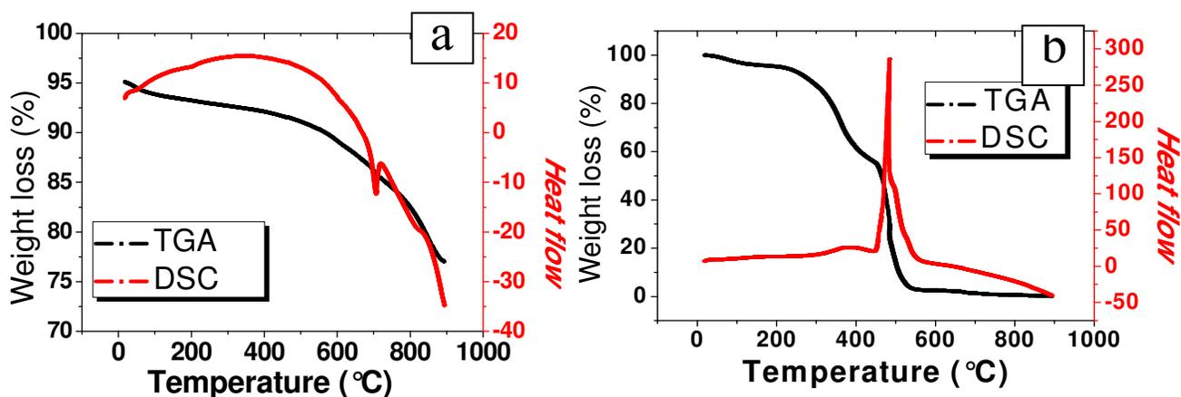
Fig.1. a) TGA and DCS analysis of  $\text{LiCO}_3$  and  $\text{CoO}$  mixture. b) TGA and DSC analysis of dry polyacrylamide gel containing  $\text{Li}^+$  and  $\text{Co}^{2+}$  cations
