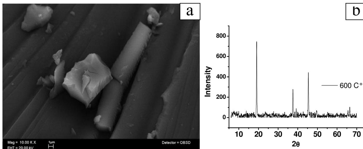
Fig.2. a) SEM images of small crystal in dry gel. The magnification used to get this image was 10.00 Kx b) XRD pattern of complex  $\text{LiCoO}_2$  that was obtained after slow heating.
