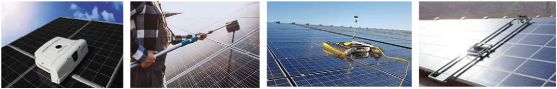
Figure 8. Illustrations of some existing solutions. From left to right: Autonomous robot, Manual tool, Installed hydraulic system, and Installed robotic system.
