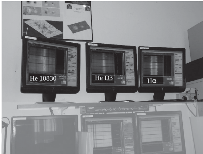
Figure 2. Observing prominences simultaneously in the 2 He lines at 587 and 1083nm plus H\alpha with THEMIS.
