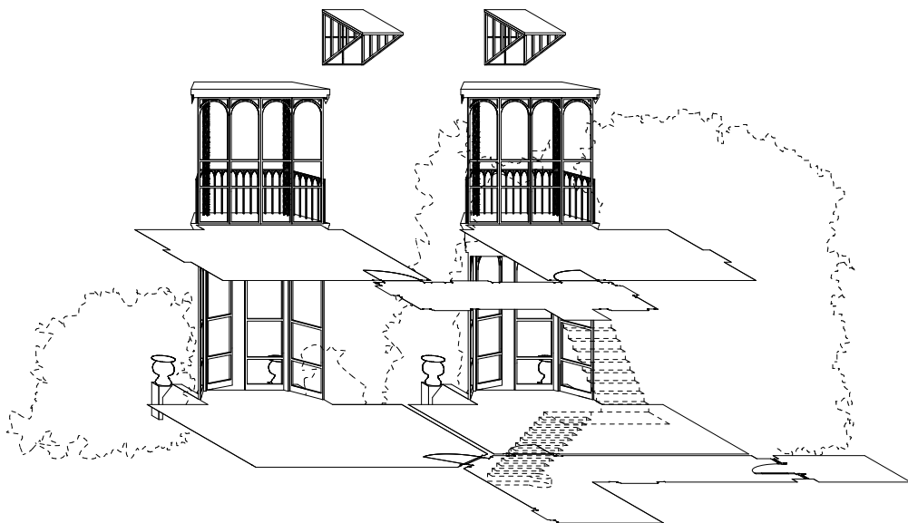
5 Analytical view of Talland House showing the pairs of bay windows, balconies, and principal rooms facing the sea. The upper left room was the nursery and upper right the parents' bedroom. The lower ground floor shows the drawing room and dining room on the left and right, respectively. The drawing, based on various sources, speculatively reconstructs the house at the time of Woolf's childhood.
