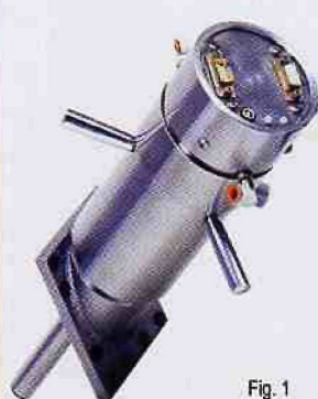
Figure 1. Photograph of SMCD spectrometer for microanalysis, which fits into the SEM column.
