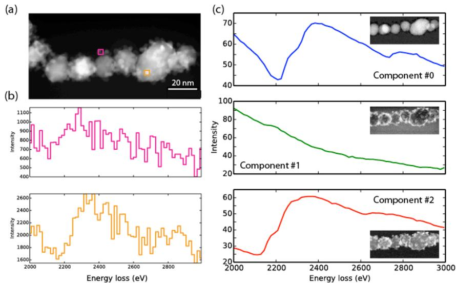
**Figure 2.** (a) TEM-EELS analysis of a AuPt nanoparticle ensemble. (b) Trace evidence of gold and platinum edges are present in the noisy raw EELS spectra. (c) ICA successfully separates the spectrally and spatially overlapping gold and platinum edges in the EELS signals present in the raw data.
