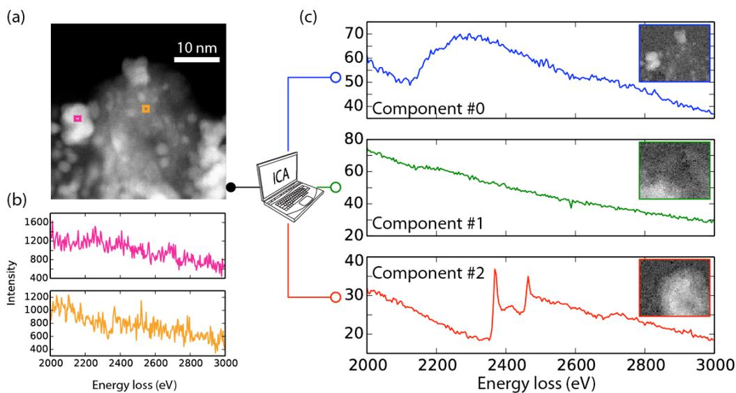
**Figure 1.** (a) TEM-EELS analysis of a fuel cell cathode material containing nano-particulate platinum and niobium oxide on a NbO<sub>x</sub>-carbon hybrid support. (b) The raw spectral data are noisy due to limited beam dose to avoid sample damage. (c) ICA finds three main components in the spectral mixture, belonging to platinum and niobium.
