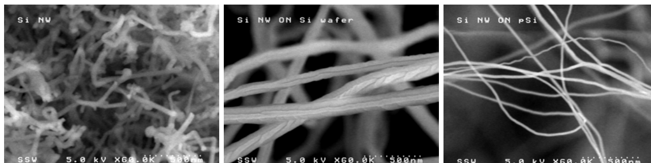
FIG. 1. SEM images of the products, from left to right: free standing SiNW condensed on the quartz tube, SiNWs collected on a Si(100) wafer and a porous silicon substrate.
