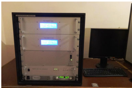
Figure 6. Transmitter of sounding pulses of the SKiYMET Meteor Radar in Kazan.
