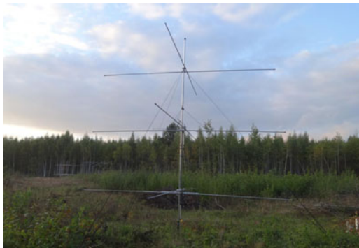
Figure 5. Transmitter antenna of the SKiYMET Meteor Radar operating in Kazan.
