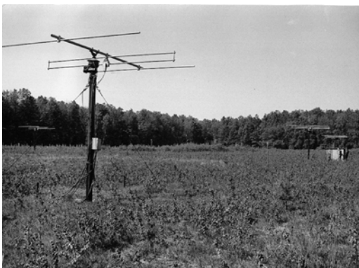
Figure 2. Phase interferometric goniometer of the “KGU-M5” radar for identification of angle of arrival of meteor radio reflections consisted of 5 Yagi antennas (photo of 1983).
