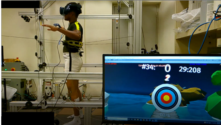
Figure 2. Subject standing in RobUST. The subject stands in the middle of the frame and a belt controlled by motors, through cables, is connected to their trunk. The subject wears a VR headset which displays a scene shown at the bottom right. The subject plays a VR catch-and-throw game using the VR wand for the catch and throw actions while receiving perturbations.
