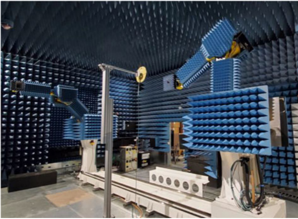
Figure 1. Dual multi-axis industrial robotic antenna measurement system, picture courtesy of Boeing.
