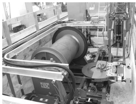
Fig. 9. Winch on the left and level wind in right foreground; cable runs around level-wind sheave to the second sheave at base of drill tower, barely visible in the background.
