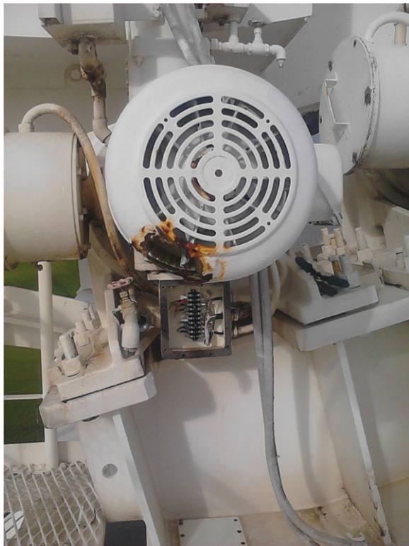
Figure 5. The state of the old motors was very poor and was considered a safety issue. (Image courtesy of Stuart Weston.)
