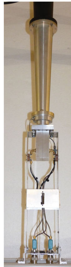
Figure 11. The C-band receiver with the new feedhorn transition unit manufactured by BAE Systems Australia. (Image courtesy of Stuart Weston.)
