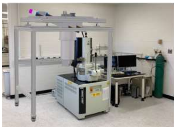
Figure 2. Left: A rendering of the dilution refrigerator with microsnout assembly coupled to the scanning electron microscope. The dilution refrigerator is the white cylinder mounted on a sliding track in the frame in the rendering. The detector microsnout protrudes from the refrigerator bottom, and in this picture it is inserted into the SEM. Right: A close-up rendering of the detector snout inside the SEM chamber, with an effective distance of 50 mm from the beam spot to the detector array chip. The sample pin stub on the yellow sample stage is shown at a working distance of 10 mm and tilt of 20°.
