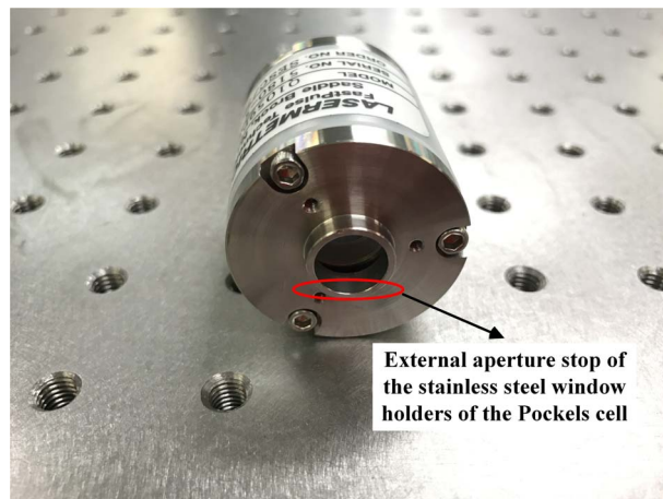
Figure 11. A photo of the PC used in the Regen. The external aperture stop of the stainless steel window holders was marked with a red circle.
