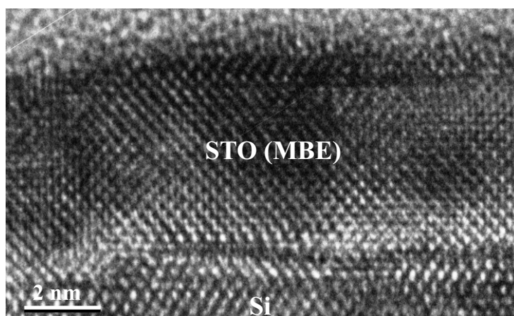
Figure 3: Cross-sectional TEM micrograph of STO (MBE) (~4.7 nm) grown on vicinal silicon (001) substrate.
