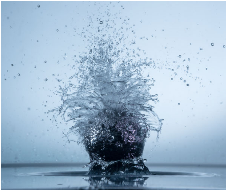
Figure 13. A 50 mm steel sphere falling through the Worthington jet originating from the collapse of a cavity created by a 38 mm hydrophobic steel sphere impacting a quiescent water pool at 2.09 \text{ m s}^{-1} . The beautiful fluid patterns observed at the surface of the sphere originate from the jet water films following the sphere curvature and crashing together at the top of the sphere.
