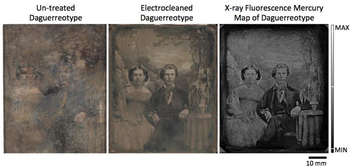
Figure 1. Before and after optical images of 19 th century daguerreotype (NGC collection; accession no. PSC 70112) and accompanying \text{Hg } \text{L}\alpha XRF map from the un-treated plate collected at the CHESS.
