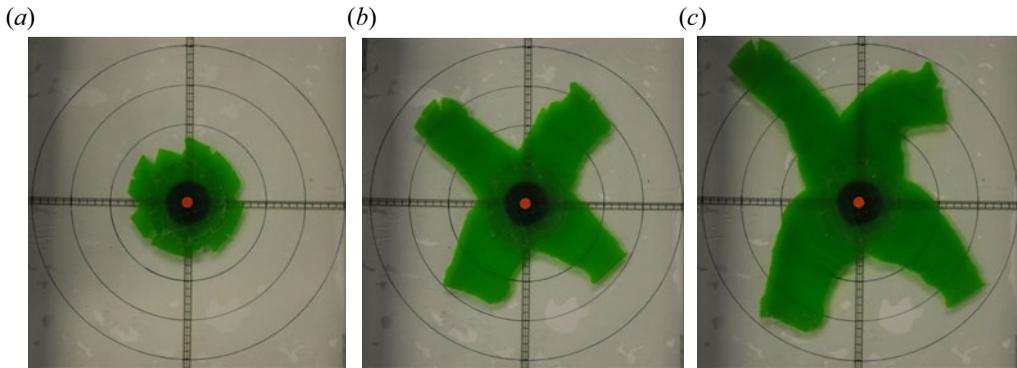
Figure 3. Sample photographs viewed from above where xanthan gum is injected at a constant flux  $Q_0 = 0.56 \text{ ml s}^{-1}$  into a Hele-Shaw cell, using disks of radius 5.5 cm and pre-formed lubrication layers of 2 mm, at times (a)  $t = 38 \text{ s}$ ; (b);  $t = 150 \text{ s}$ ; and (c)  $t = 258 \text{ s}$ .
