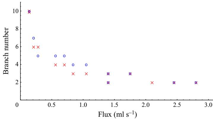
Figure 6. Branch number plotted against flux for the experimental set-ups using disks of radius 5.5 cm, where the data points  $\times$  (red) and  $\circ$  (blue) correspond to 2 and 1 mm lubrication layers, respectively. The number of branches decreases with increasing flux, and between the two sets of experiments, there is a difference of at most one branch at a given flux. Repeated experiments are offset slightly.
