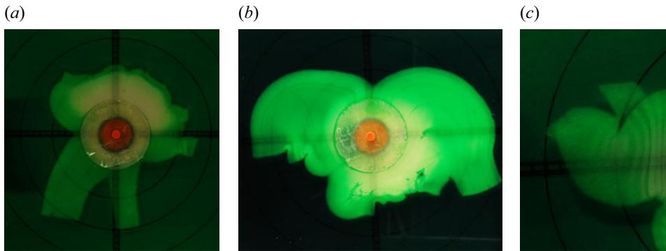
Figure 9. Sample photographs viewed from above for three different experiments using disks of radius 5.5 cm and pre-formed lubrication layers of 1 mm where (a) the output flux is  $1.4 \text{ ml s}^{-1}$ ; (b) the output flux is  $2.8 \text{ ml s}^{-1}$ ; and (c) a branch of an experiment using a flux of  $1.05 \text{ ml s}^{-1}$  is shown. Note the vertical striations, indicating out-of-plane folds in the extruded fluid.
