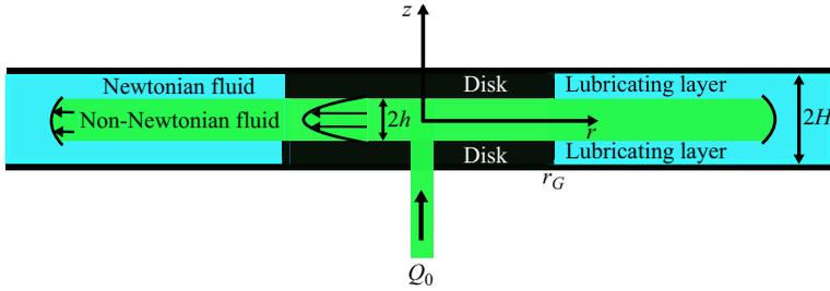
Figure 1. Side view of the axisymmetric injection of a shear-thinning fluid that fills the gap of size  $2h$  between two disks completely for  $r < r_G$ , and is confined between two lubricating layers of Newtonian fluid in the region  $r > r_G$ , where  $r_G$  is the radius of the disks.
