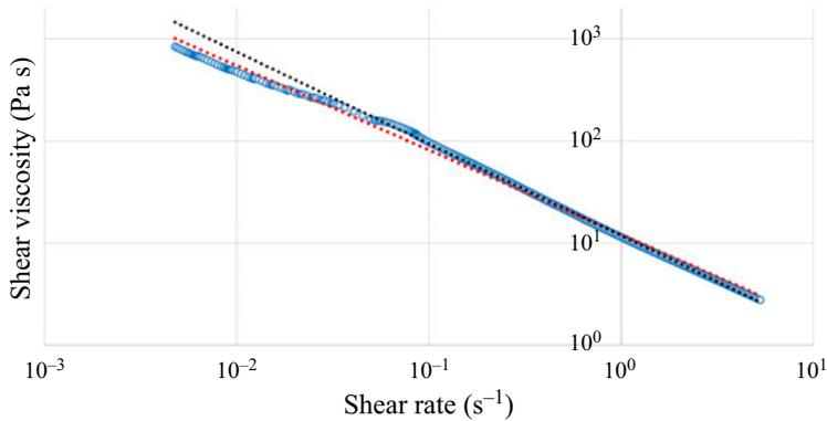
Figure 10. Shear viscosity (Pa s) versus shear rate ( $\text{s}^{-1}$ ). The black-dotted and red-dotted lines correspond to the approximations with  $n$  and  $m$  values given by (A1) and (A2), respectively.
