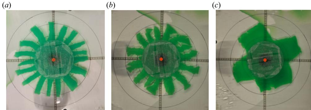
Figure 7. Sample photographs viewed from above for three different experiments using disks of radius 8 cm and pre-formed lubrication layers of 2 mm, where (a) the output flux is  $0.14 \text{ ml s}^{-1}$ ; (b) the output flux is  $0.28 \text{ ml s}^{-1}$ ; and (c) the output flux is  $1.75 \text{ ml s}^{-1}$ .
