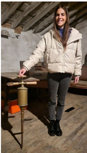
Figure 11. Maria Pinheiro da Veiga shows the tool used to inject CS 2 deep into the root area of a vine to kill phylloxera. Her great-great-grandfather Joaquim Pinheiro de Azevedo Leite Pereira, 10th Lord of Casa do Santo, initiated the fight against phylloxera and became known as the ‘saviour of the Douro’ (photo: SKE).
