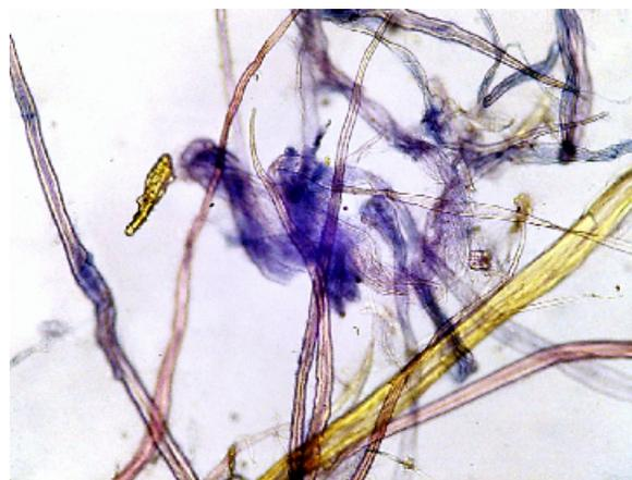
FIG. 2. Herzberg stain of paper towel fibers indicating chemical and mechanical pulp. 40 X
