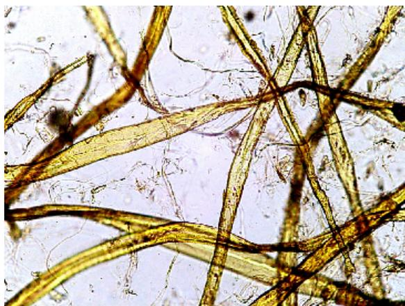
FIG. 1. Graff "C" stain of thermo-mechanical pulp with high lignin content. 40X
