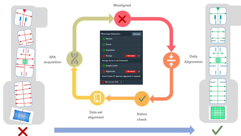
Figure 1. Automatic Microscope Status Checks and Alignments during Daily SPA Routine
