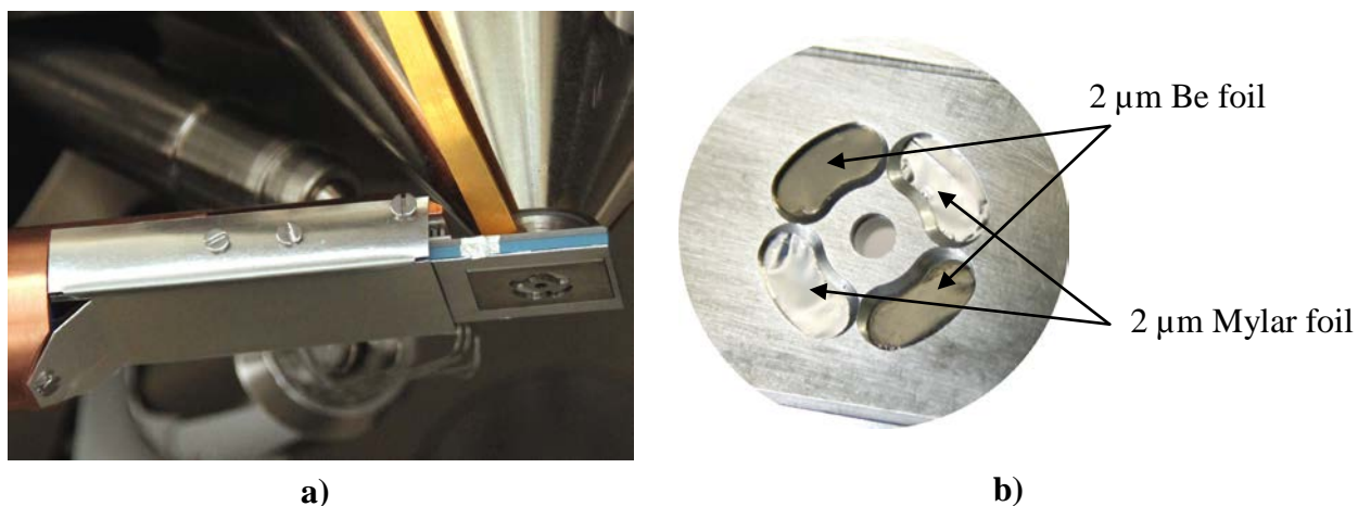
Fig.2. a) The annular pole piece EDX detector “Rococo2” inside the SEM and b) a view at the top of the detector showing the collimator with a filter combination of 2 \mu m Be and 2 \mu m Mylar.
