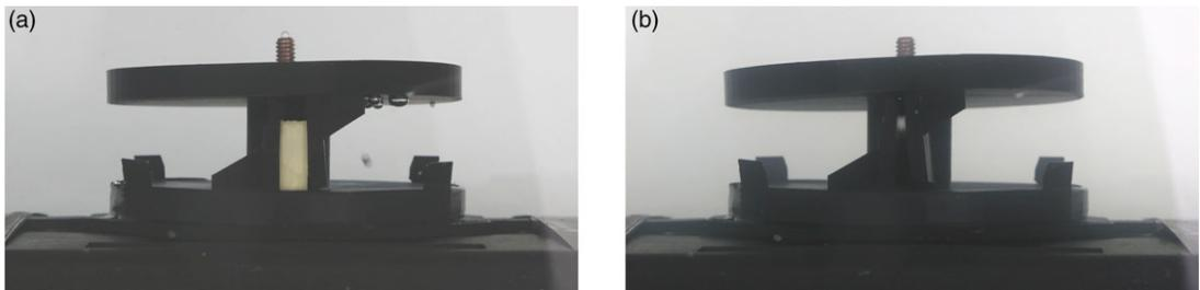
**Figure 5.** Twist test (a) before and (b) after the test which utilized PVA as the resorbable material. The insert is the off-white section visible in the center of the mechanism in (a).
