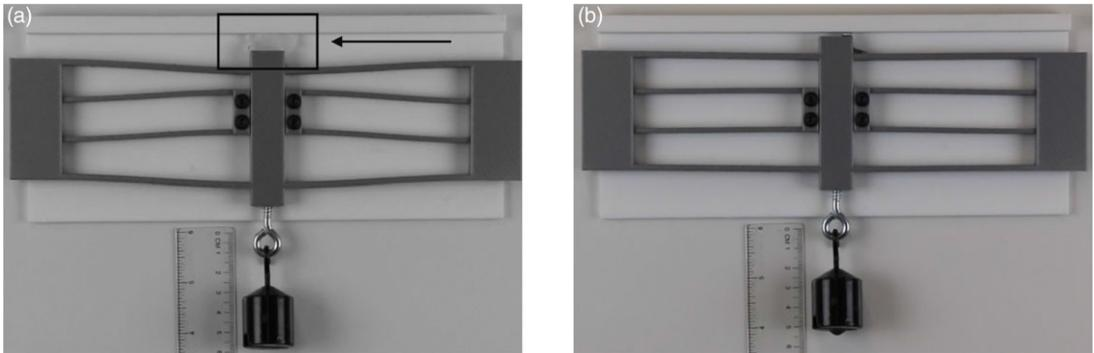
**Figure 8.** Linear test (a) before and (b) after, utilizing ice as the resorbable material. The ice is indicated by an arrow and box in (a).
