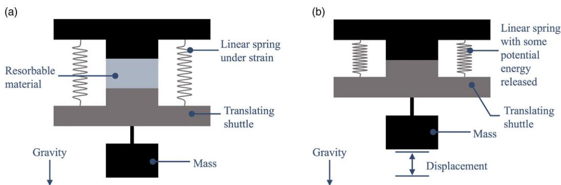
**Figure 7.** Schematic illustrating the basic concept of Mechanism 2. (a) The linear springs have stored potential energy. (b) The potential energy is released as the resorbable material dissolves and lifts the weight.
