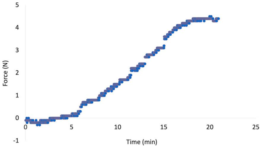
**Figure 14.** Force versus time data received from test 3. This data shows a clear increase in force over time as the inserts dissolve.
