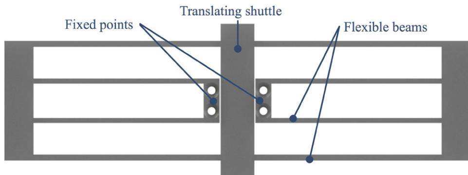
**Figure 6.** Rendering of the folded-beam suspension.
