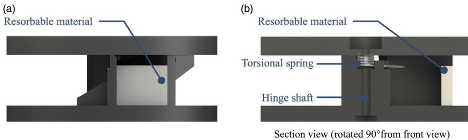
**Figure 4.** Renderings of the twist design in a (a) front view and (b) section view (rotated  $90^\circ$  from front view). The white piece of resorbable material is visible, as well as the torsional spring which provides the actuation energy.
