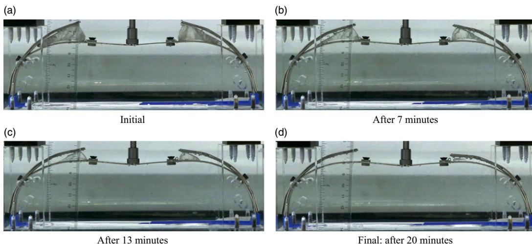
**Figure 11.** Pectus bar throughout resorption process from test 3: Aluminum mechanism with rock salt inserts. The rock salt is visible in (a) on each upper side of the insert.
