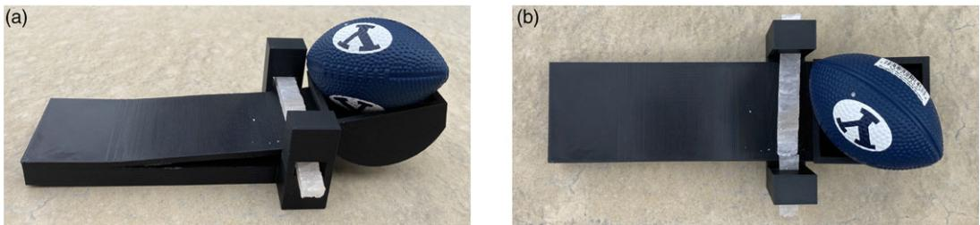
Figure 16. The catapult with the arm restrained by a bar of rock salt. (a) Angled view. (b) Top view.
