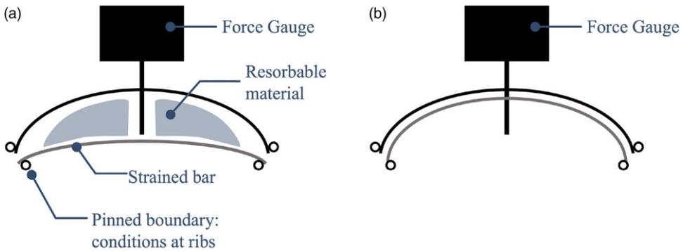
**Figure 12.** Schematic illustrating the basic concept of Mechanism 3. (a) The linear springs have stored potential energy. (b) The potential energy is released as the resorbable material dissolves.
