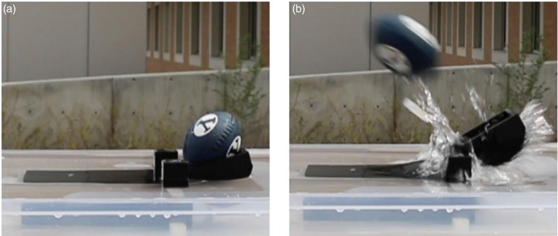
**Figure 18.** *Catapult test (a) before and (b) after the test. Rock salt was used as the resorbable material. Refer to Fig. 16 for a better visualization of the insert in (a); in (b), the shattered pieces of insert are visible behind the splash.*
