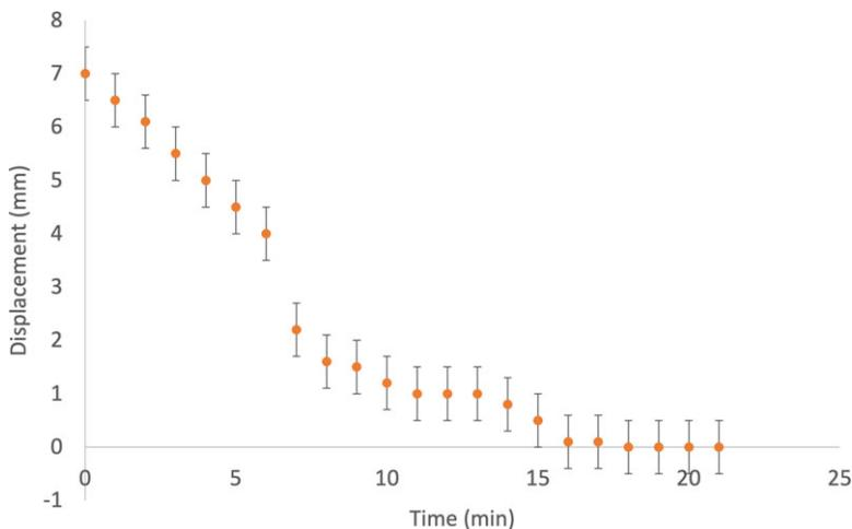
**Figure 9.** Displacement versus time data received from the folded-beam suspension test, including bars of uncertainty. This data shows a clear, nonlinear increase in displacement over time as the inserts dissolved.
