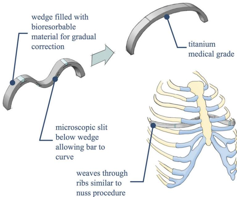
**Figure 13.** An initial conceptual design for the corrective bar. The design changed somewhat before the final iteration tested in this work, but the concepts of surgical insertion and gradual correction are the same.
