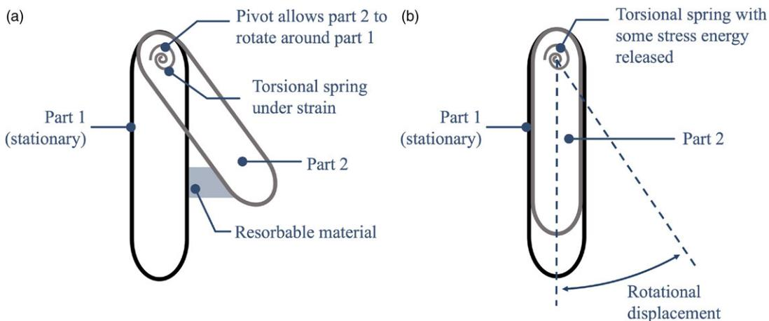
**Figure 2.** Schematic of the basic concept of Mechanism 1. Part 2 rotates relative to part 1 as the resorbable material dissolves. (a) The two parts are connected at a pivot (hinge) with a torsional spring that stores potential energy which is (b) gradually released as the resorbable material dissolves.
