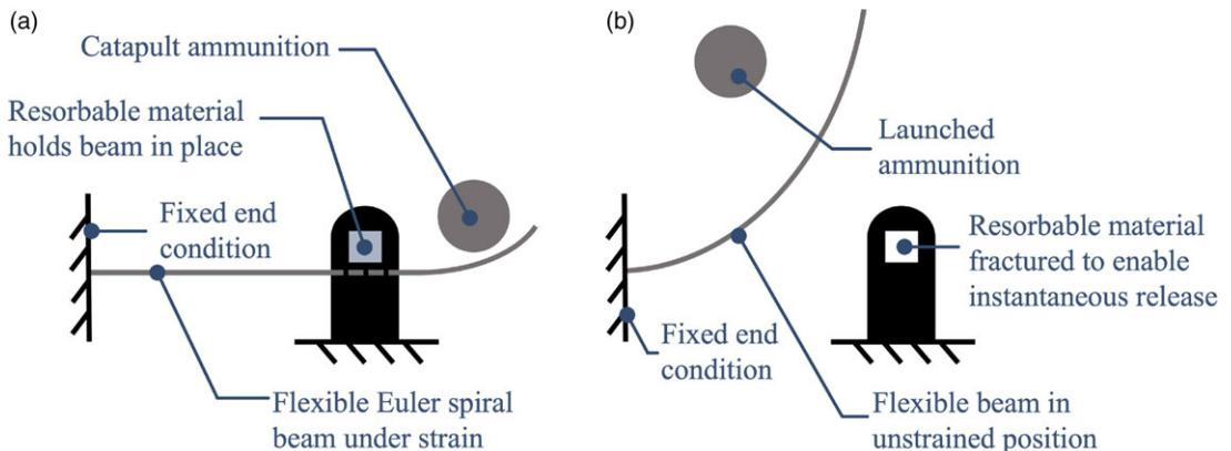
Figure 17. Schematic illustrating the basic concept of Mechanism 4. (a) The Euler spiral beam is held under strain by the resorbable material. (b) When the resorbable material fractures, the strain energy is released and the ammunition is launched.
