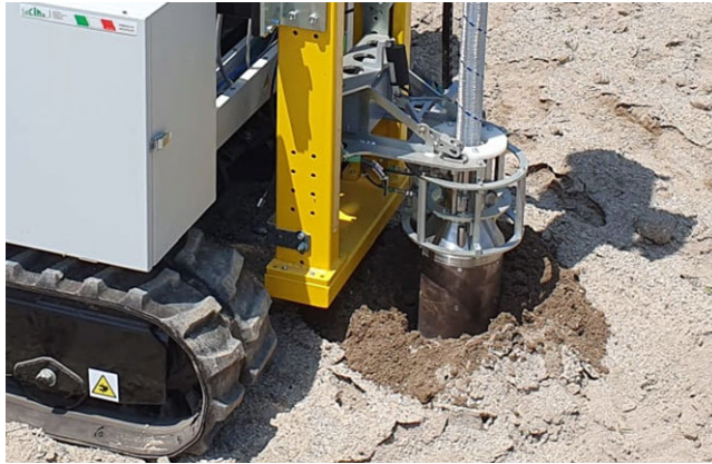
Figure 2. Snapshot of the ROBILAUT robot during drilling, a mechanical sampling mechanics is embed in the head and allows for the required quartering task.
