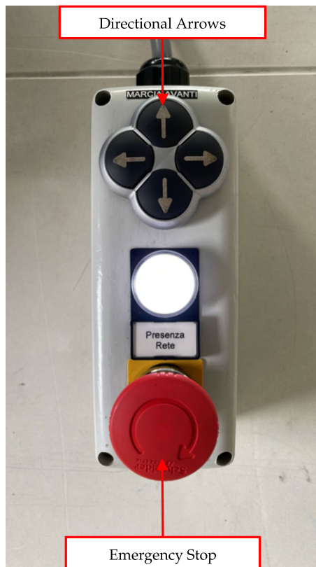
Figure 6. Joystick for the manual movement of the ROBILAUT vehicle equipped with emergency button for safety reasons.
