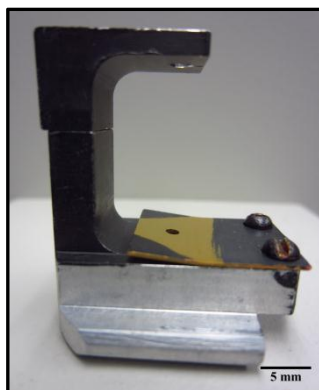
FIG. 1: Updated simultaneous BF and DF STEM-IN-SEM specimen holder for Hitachi S-4300SE/N.
