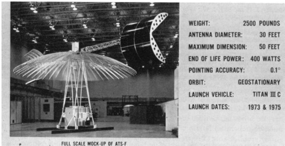
Fig. 9. ATS-F and G characteristics. Full scale mock-up of ATS-F.
