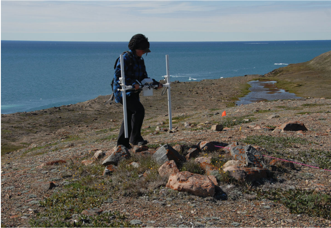
FIGURE 2. Magnetometer survey (Bartington Grad 601 Dual Sensor Fluxgate Gradiometer) on Banks Island showing rock features common on the surface of Arctic sites. Note opened meat cache in the foreground.
