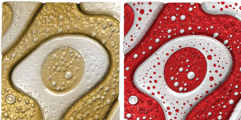
Figure 4: Dynamic mode images of a blend of polystyrene/poly(styrene-butadiene-styrene): (Left) topographic image and (right) phase image.
