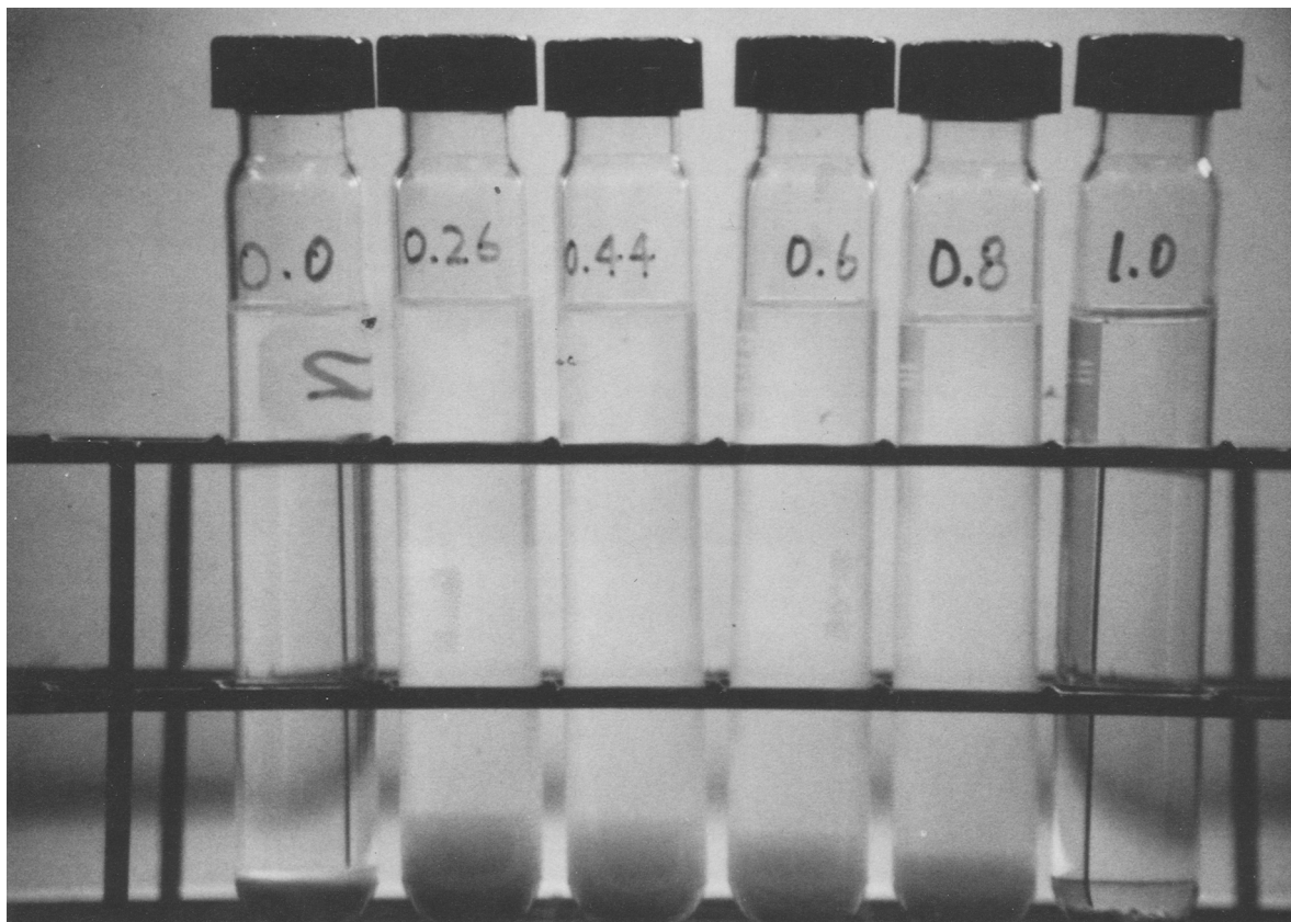
Figure 9. Benzylammonium-montmorillonite dispersed in binary mixtures prepared from water and acetonitrile. The numbers on the tubes indicate the mole fraction of water. The tubes were photographed 3 mo after initial mixing.
