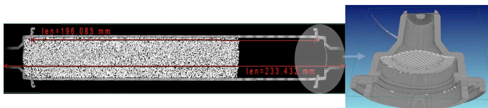
Figure 3. Results of a 15 minute CT scan of cartridge device where both dimensional information relative to specifications from the 2D radiographs and weld morphology from the 3D reconstruction were acquired.
