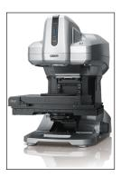
The VR-3000 is a non-contact, wide-area 3D measurement microscope that performs sub-micron resolution scanning in seconds. After scanning, the microscope creates a 3D model of the sample, which can be analyzed for form, contour, flatness, warpage, curvature, line roughness (ISO 4287:1997), surface roughness (ISO 25178), and more. Scans can be directly overlaid against 3D computer-aided design (CAD) models to visualize and quantify surface shape
