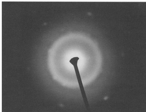
Figure 3. Selected area electron diffraction pattern obtained from an aggregate of small particles in NF 30-40 .
