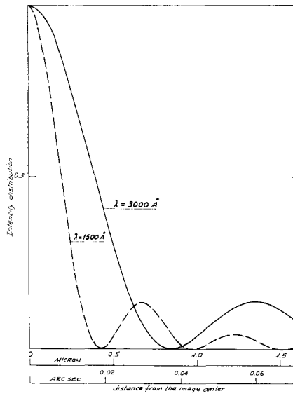
Fig. 2. The point spread function on the axis at the focal plane.
