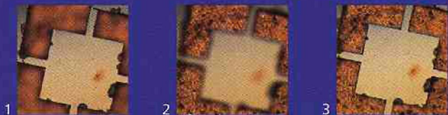
1 2 3 4 1000 fps are captured to identify sharp pixels in different depths of field (1 & 2) prior to being interpolated into a 30 fps "all-in-focus" video (3)
