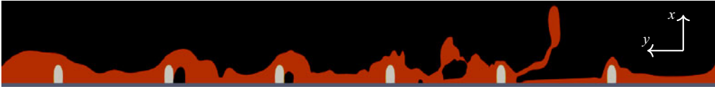
Figure 8. Snapshot of the volume fraction field close to the inlet for an evaporating falling film (Case M3 with Ka = 488 , Re = 215 ) on a modified surface. The liquid flows from left to right with the domain inlet at the left-hand edge. Note that the horizontal axis (but not the vertical) is scaled by 0.5 for visualisation purposes, thus altering the aspect ratio. The black colour represents the gas phase, red the liquid and grey is the surface modifications. Sputtering events (detachment of liquid ligaments) and entrainment of bubbles appear at this Re number and become even more frequent at higher values of Re .
