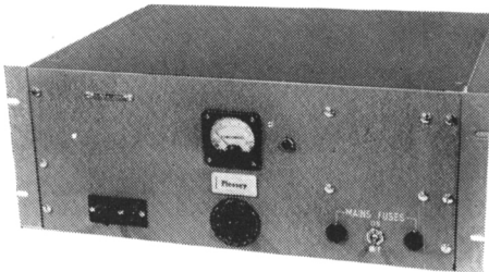
PV 14 Wide band aerial amplifier enabling up to ten communication receivers to be operated from one common aerial system. Handles large signal inputs without overloading or cross-talk becoming excessive. Low noise factor. Available for 75 or 600 ohm inputs. Designed to International Aeradio Specification.
