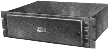
PR 51 H.F. Receiver for high quality reception of R/T M.C.W. and C.W. in the 2-20 Mc/s band. Temperature compensated R.F. and oscillator circuits with crystal control or free tuning as required. Simple to maintain as valves and all major components are readily accessible. Fitted with automatic channel indication and muting control. Local or remote control. Designed to International Aeradio Specification.
