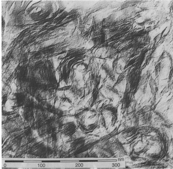
Figure 3. TEM lattice-fringe image of smectite from 512 mbsf. Curved packets commonly form circular units (inferred to be spherical in three dimensions) that result from progressive alteration toward the core of glass shards, with smectite layers wrapping around shards (not shown).
