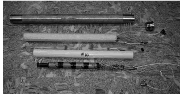
Fig. 4. Probe components. The unit at the bottom consists of the transmitting coil, batteries, tiltmeter, microprocessor and pressure transducer. Above it is the same type of unit after being cast in epoxy within a plastic tube. Shown above this tube is another after it has been wrapped in foam, which will enable it to fit smoothly into the stainless pressure casing (0.61 m long) at the top. Springs and more foam at the ends are not shown.
