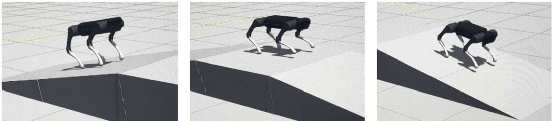
Figure 18. Snapshots of the quadruped robot going upslope (left), platform motion (center), and downslope (right).
