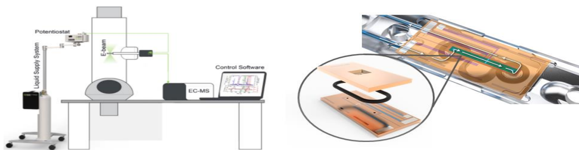
Figure 1. (Left) Schematic overview of the integrated Stream LPEM-ECMS system. (Right) Render of the Stream liquid biasing holder with an inserted Nano-Cell and a flow path of the liquid; the top chip is made transparent for observation. The inset shows the bottom and the top chips of the Nano-Cell with an O-ring.
